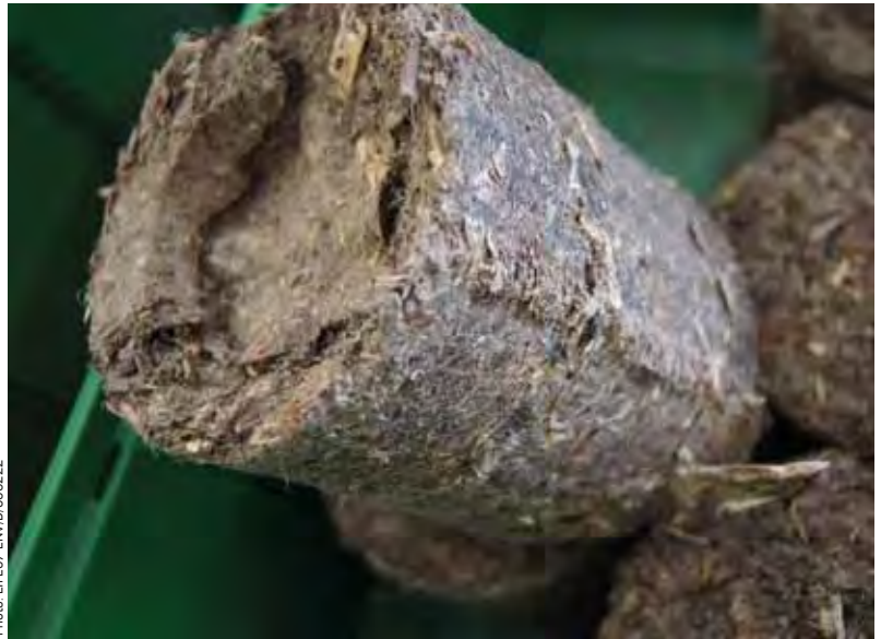
The project converted late-harvest grass into solid biomass briquettes
