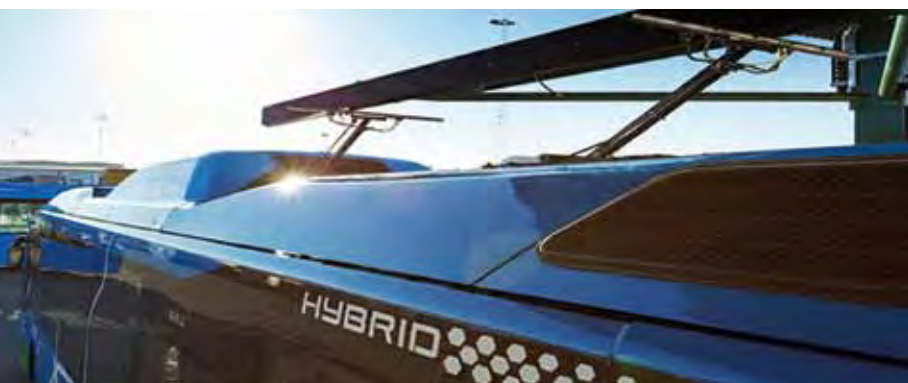
The plug-in hybrid buses can be charged rapidly at each end of the route
